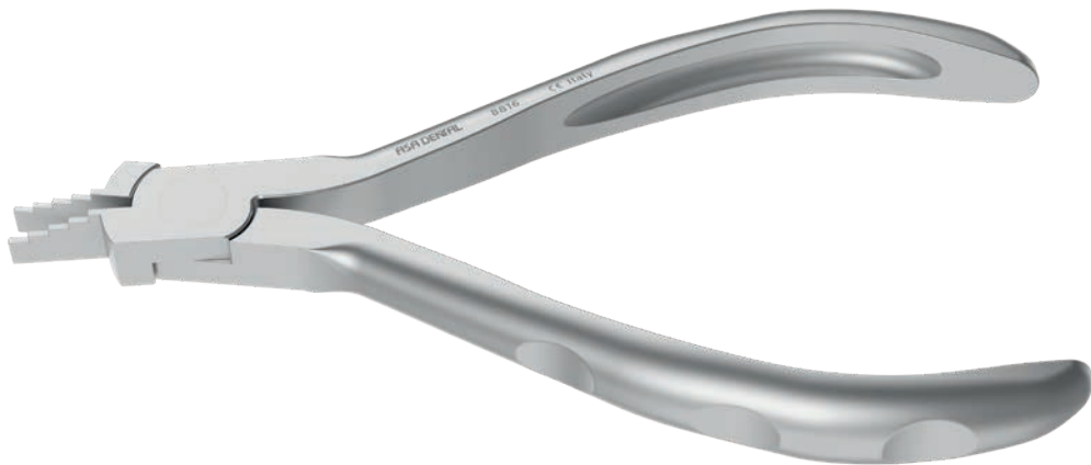
Nance precision pliers 8816 For precise forming of loops in 4 different lengths: 3, 4, 5 and 6 mm. A groove at the base aids in closing loops. Wire size: max. 0.70 mm (0.028")
