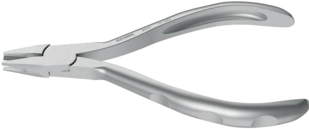
V-stop pliers 8830 Designed to create V-bends in archwires, including those in nickel titanium, and prevent archwire from travelling. Wire size: max. 0.70 mm (0.028")
