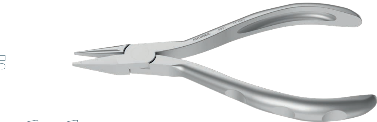
bird beak pliers 8821 Light wire bird-beak pliers with a groove. The longer conical beak facilitates the creation of precise loops. The groove makes it easy to locate and duplicate loops. Wire size: max. 0.70 mm (0.028")
