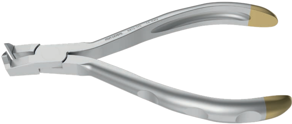
universal distal-end-cutter, no hold 8813-1TC Mini universal distal end cutter, without safety hold. Cuts flush to the bracket or buccal tube. Wire size: max. 0.56 mm x 0.70 mm (0.022" x 0.028")
