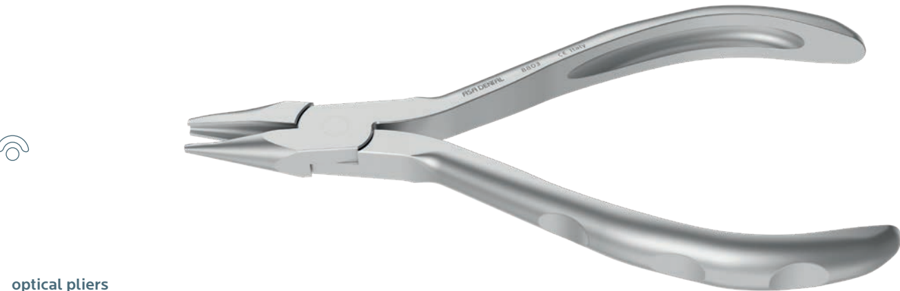
optical pliers 8803 Pliers with a groove, excellent for forming helical closing loops and wire bending of round and rectangular wire. Wire size: max. 0.70 mm (0.028")
